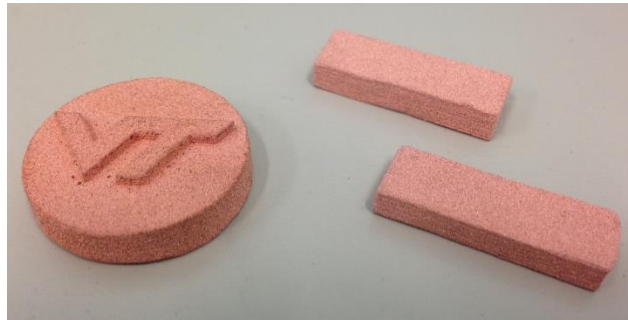
Figure 6. Sintered copper part samples (AcuPowder 153A copper powder sintered in pure hydrogen at 1000 °C for 8 hours)
