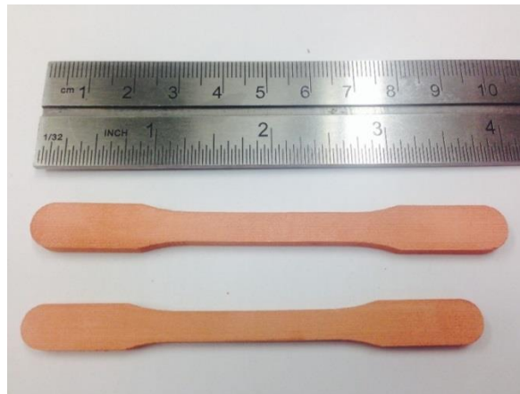
Figure 12. Tensile test specimen: sintered at 1060 °C (top) sintered at 1080 °C (bottom)
