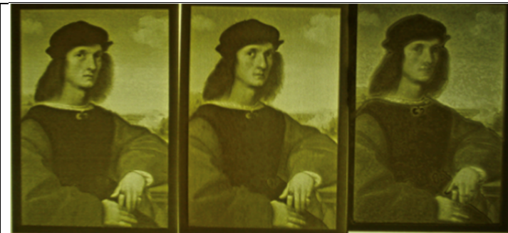
Figure 6: Polyamide 12 lithophanes laser sintered with 0.102 mm of layer thickness built in the ZX, YZ, and XY planes from left to the right. The size of lithophanes was 127 mm by 76 mm, with maximum plate thickness equal to 3.8 mm. Lithophane photos were captured using white light box illumination.
