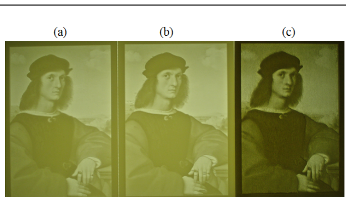
Figure 11: SL lithophanes built (a) in the XY plane; (b) built in the ZY plane; and (c) LS lithophane built in the ZY plane. The maximum plate thickness for each was 5 mm. Lithophane
