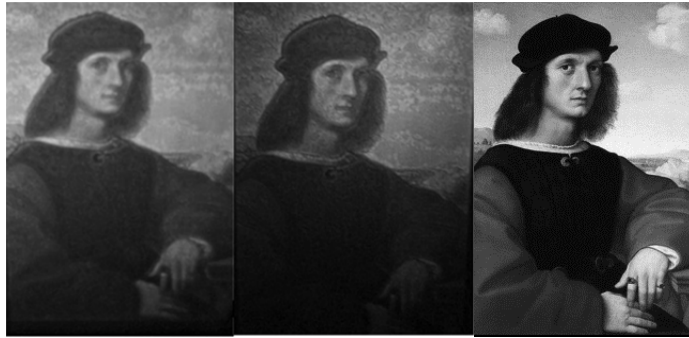
Fig 3: Gray-scale processed laser sintered polyamide 12 3.81mm thickness lithophanes under different monochromatic light: green (left), yellow (center). On the right is the initial digital image used to create the lithophanes.
