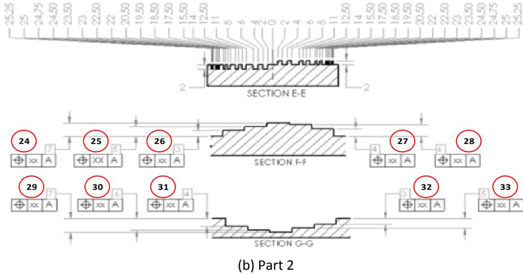
Fig.3 Geometrical characteristics of NIST standard test part [15]
