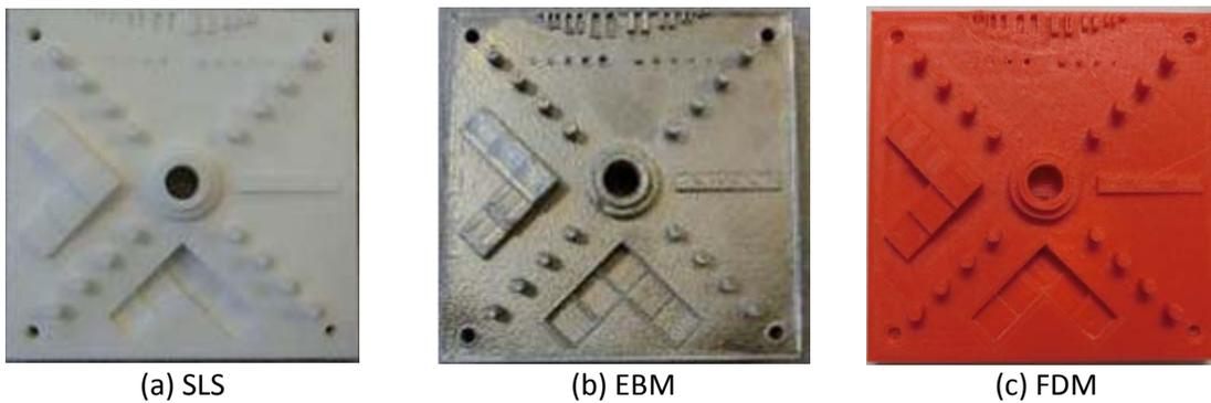
Fig.4 Samples of NIST test part
