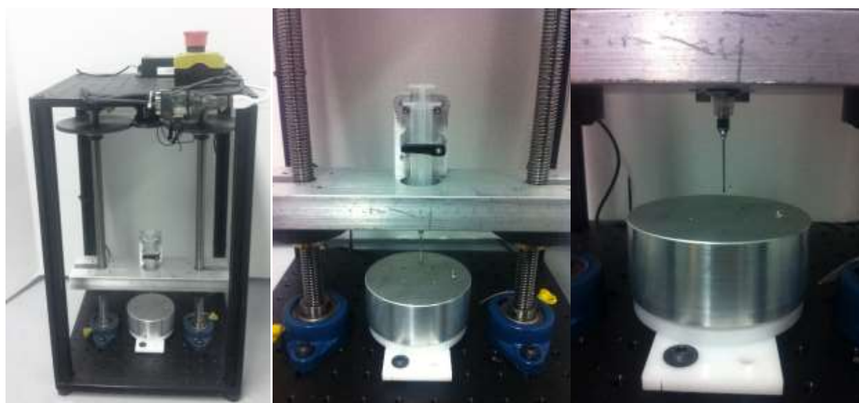
Figure 2: A freeloader system (a) was modified to include a 10CC BD syringe (b) and a compression load cell (c) to allow for materials testing.
