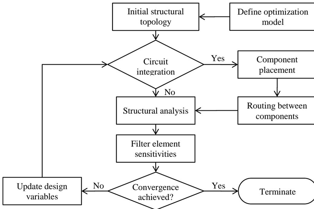
Figure 7: Flowchart showing the coupled optimization procedure
