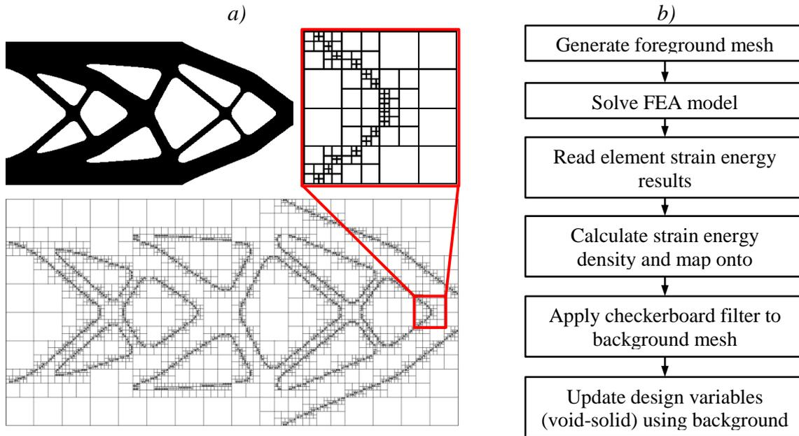
Figure 8: a) An octree decomposed topology used for analysis,
