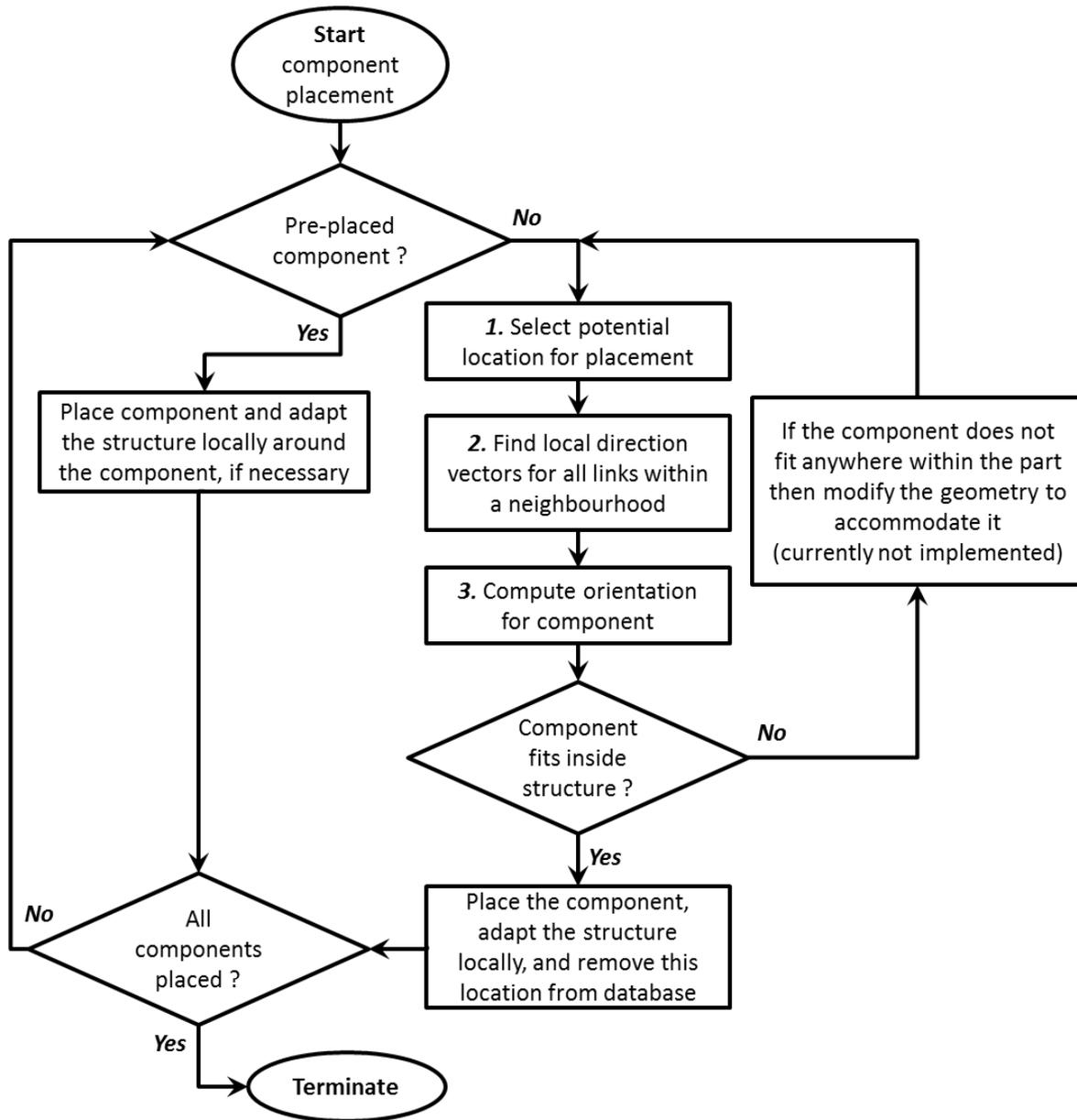
Figure 6: The placement methodology
