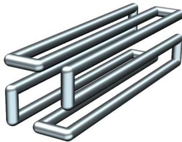
*Figure 10 – Example of design freedom in creating a compact 3D strain gauge to be placed in thin structural members.*
