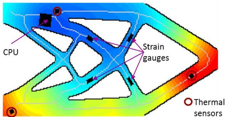
Figure 5: An example demonstrating component placement based on performance measures.
