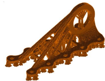
Figure 10: FE mesh of a bionic aerospace bracket
