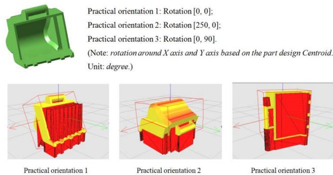
Figure 14, Practical alternative orientation set for a part.
