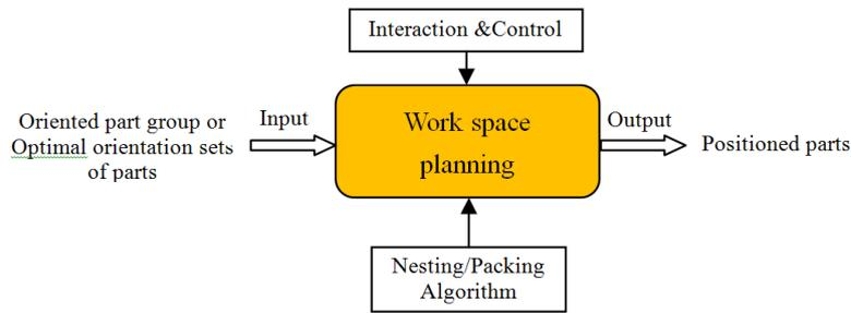
Figure 8, Functional module for 'Work space planning'.
