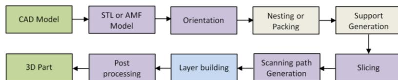
Figure 2, General processing chain of AM (‘micro level’; ‘one-way’ information flow).
