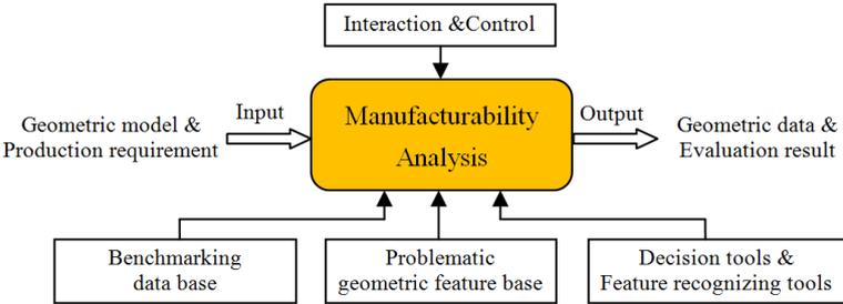
Figure 4, Functional module for ‘Manufacturability Analysis’.
