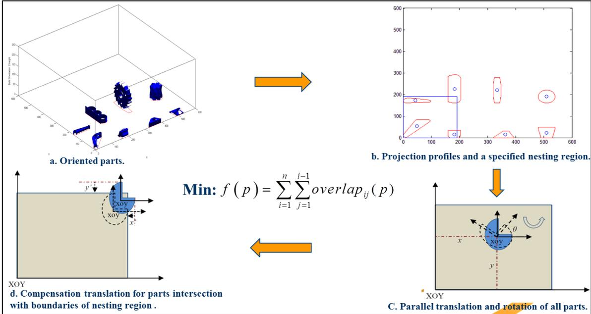
Figure 12, A proposed parallel 2-D nesting method.
