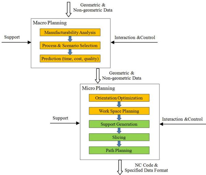
Figure 3, Main planning tasks of process planning in Multi-part production context.
