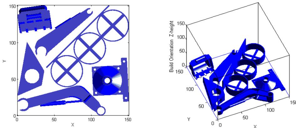
Figure 18, Nesting result for the six oriented parts.
