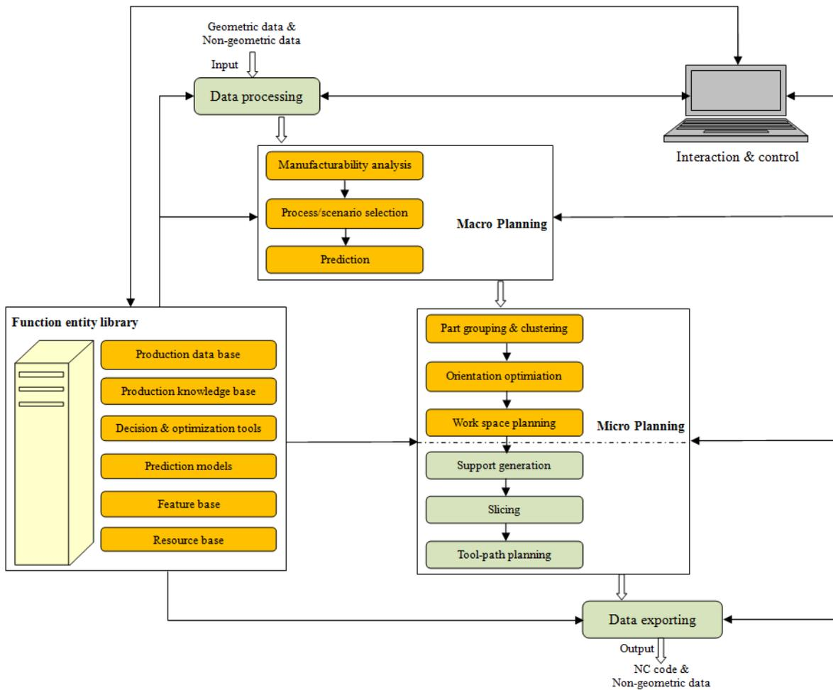
Figure 10, AM feature and knowledge based systematic process planning framework for AM in Multi-part production context.
