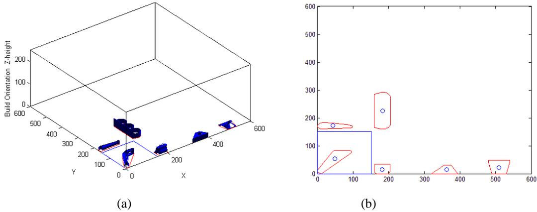
Figure 16, (a), Six parts to be nested and a specified nesting region; (b), Convex approximate polygons.
