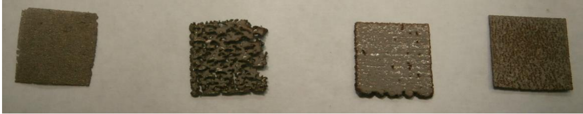
Figure 14: Failure modes from left to right: lack of fusion, balling, overmelting, and warpage out of the recoater plane.
