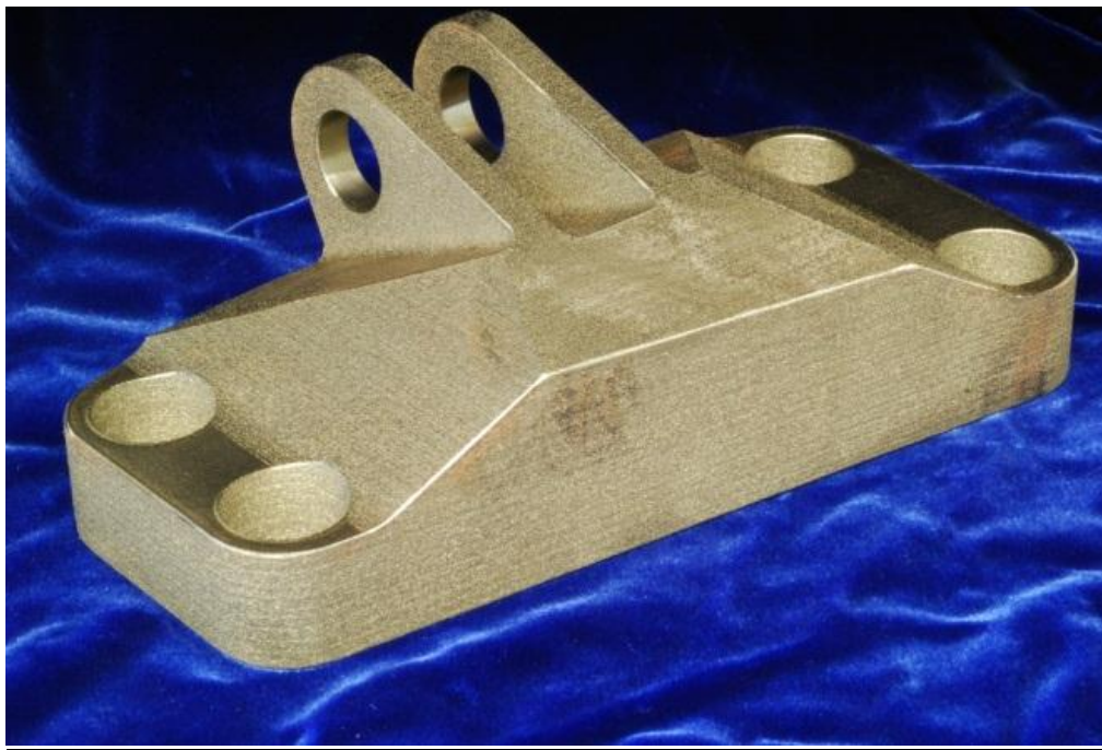
Figure 1. The original bracket design. This part was machined from titanium bar stock and weighed 4 lb.
