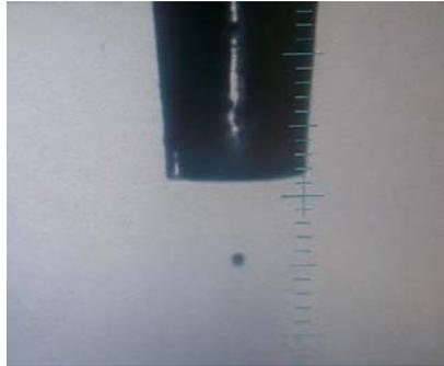
Figure 3. An optical micrograph taken with a stroboscope demonstrating optimised droplet formation.
