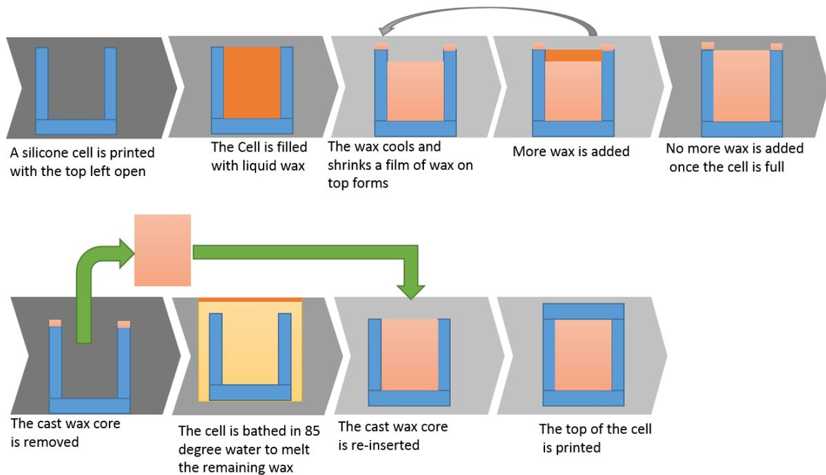
**Figure 2:** The method for producing wax actuators with Solid Freeform Fabrication and casting contains nine steps. The wax is poured into the printed cell which acts as the mold for the first 5 steps. The cell is cleaned in steps 5 through 8 and finished in step 9.
