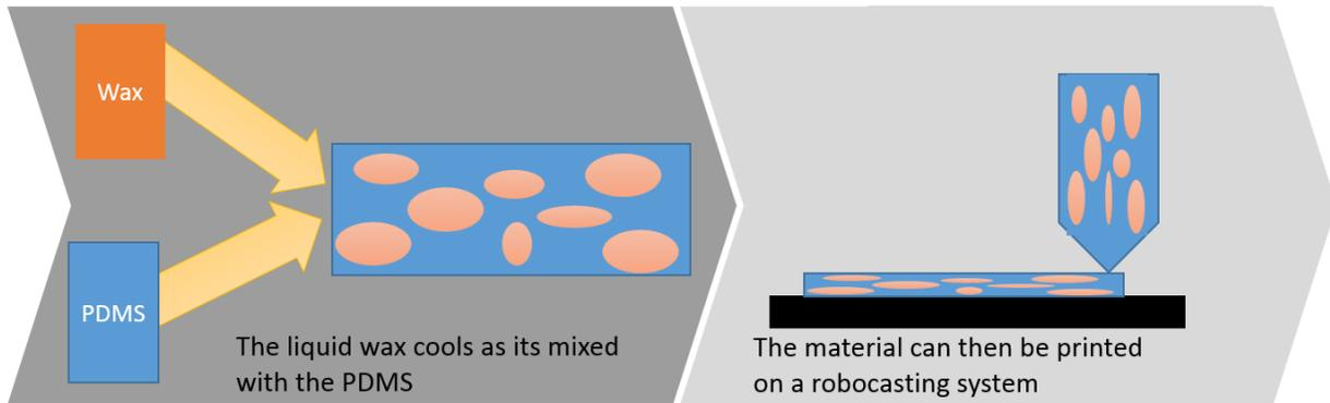
**Figure 4:** The liquid wax (bright orange) is mixed with the PDMS mechanically and rapidly. While mixing the wax solidifies. The PDMS-wax material must be printed quickly before for PDMS pot-life ends and the viscosity begins to change.
