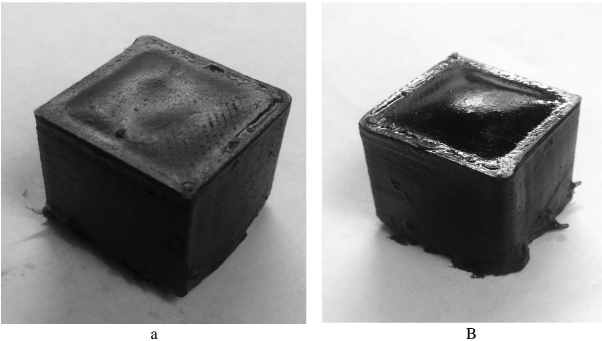
**Figure 3:** a sealed cell after 1 cycle of heating (a) can be reheated, causing expansion in the cell. (b) the cell will find the lowest energy state for the new internal volume. A thin side can direct the expansion into that a direction (b)
