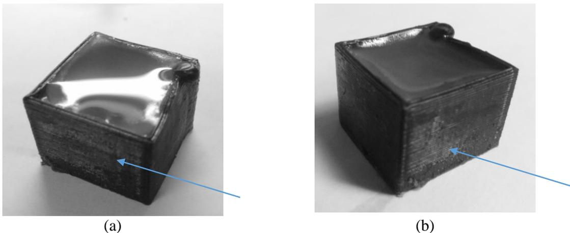
**Figure 1:** a cell filled with liquid wax (a) develops a depression (b) as it starts to cool. Overfilling errors and spills can cause wax films to form on the silicone surfaces as seen in the areas highlighted with the blue arrows
