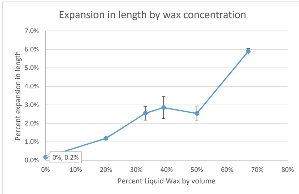
**Figure 6:** Increasing the percentage wax in the material increases the amount the material expands when heated. There is an unexpected decrease in the percentage of expansion between 40% and 50% of wax by volume. The cause of this decrease is unknown.
