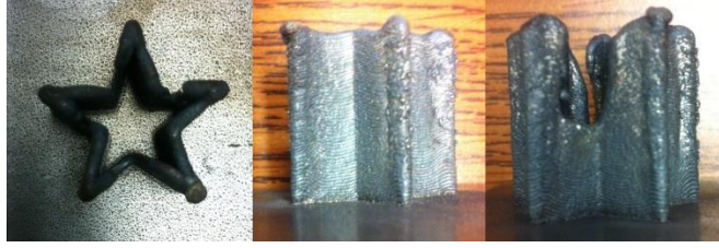
Figure 1. Photograph of a failed constant process parameter deposition.
