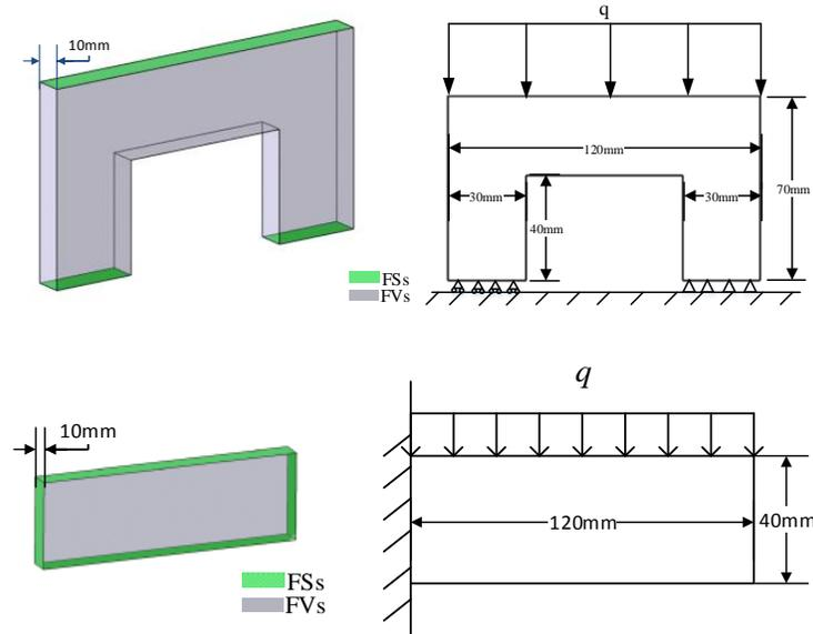
**Figure 9** The input FSs and FVs of two design cases
