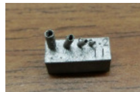
Fig. 7 Fabricated samples (100W, 500mm/s, contour + edge)
