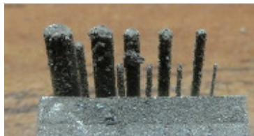
Fig. 8 Worn parts (80W, 500mm/s, contour + hatch)
