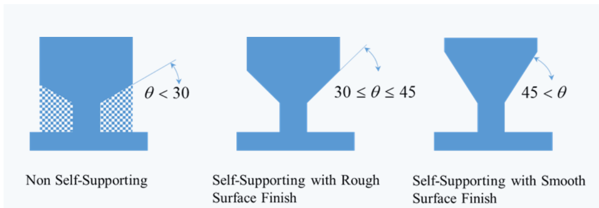
Fig. 2 An example set of commercial design guidelines introduced for the case study [14]
