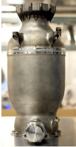
(b) SpaceX combustion chamber [2]
