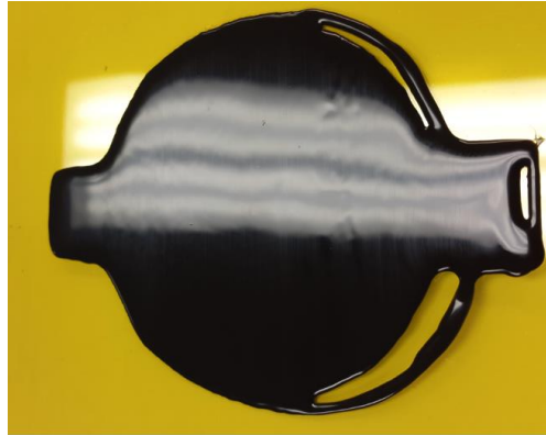
Figure 6. A good quality silicone elastomer film with extra areas.
