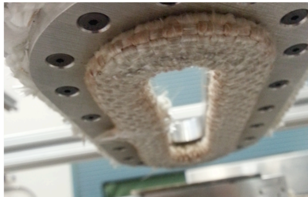
Figure 6 - High temperature seal after 3000 cycles at 330C
