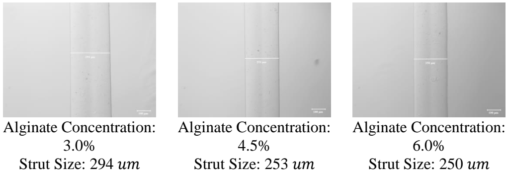
Figure 5. Strut formability in regarding to alginate concentration (viscosity): the alginate concentration examined were 3.0%, 4.5% and 6.0% (w/w). The strut size were 288 \mu\text{m} , 250.20 \mu\text{m} and 250.20 \mu\text{m} with standard error of 4.06 \mu\text{m} , 2.59 \mu\text{m} and 2.59 \mu\text{m} respectively.
