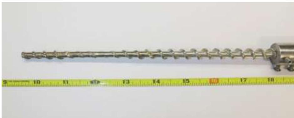
Figure 4: Auger worn-out during experiment
