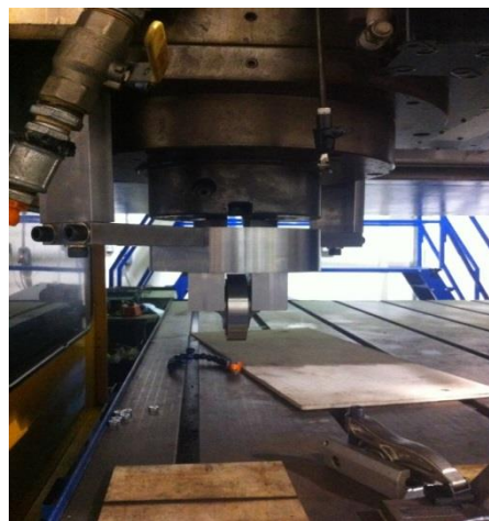
Figure 9 Rolling rig added as an additional feature to CNC system
