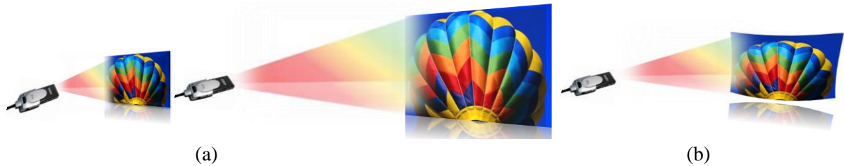
Figure 2. Laser Projector unique properties: (a) Stays focus when changing focal length; (b) Project on any shape surface
