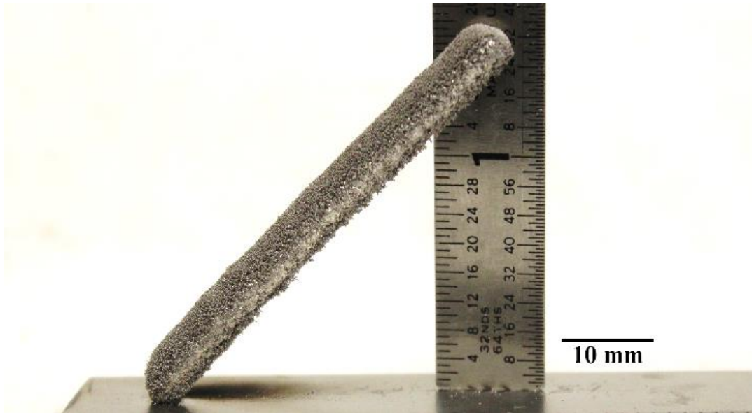
Figure 4: Forty-five degree overhanging structure.
