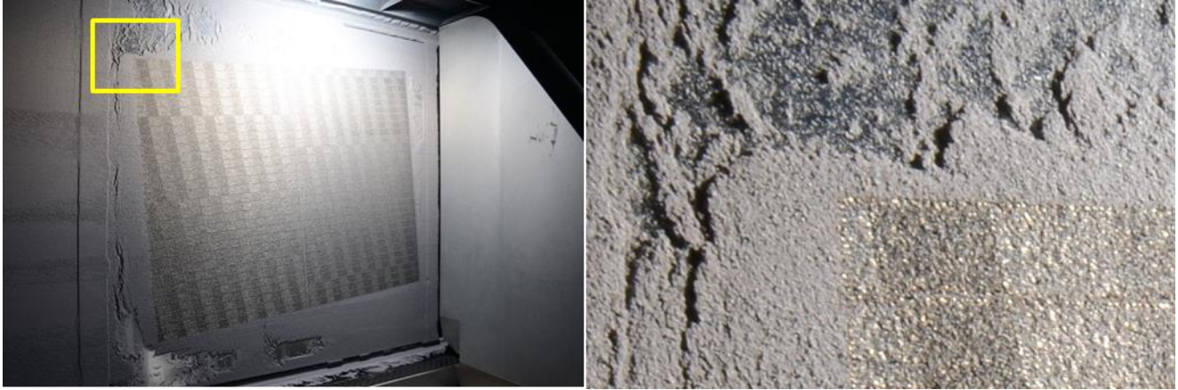
Figure 4. Image highlighting an example of powder shorting within the process chamber.
