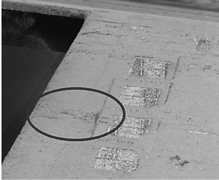
Figure 6. Image taken during PBFAM build highlighting powder flicking due to recoater blade spring-back.
