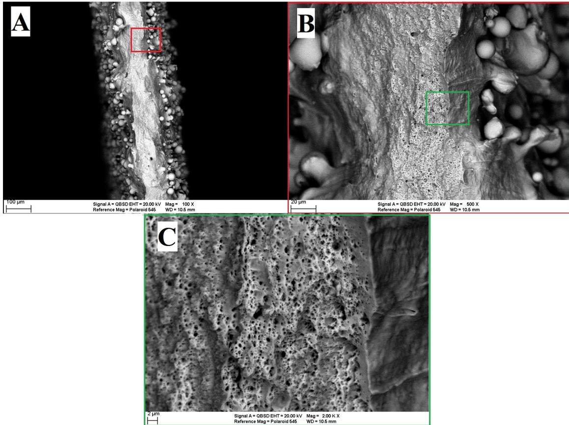
Figure 16: Fractography of 0.25 mm Sample with Compensated Scan Pattern at x100 (A), x500 (B), and x2000 (C) Showing Ductile Failure
