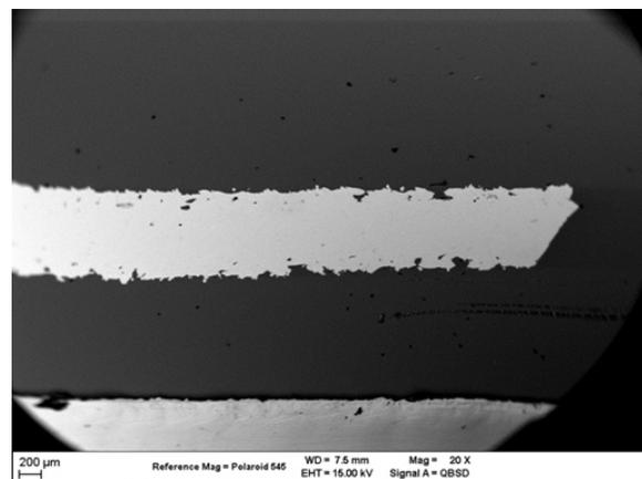
Figure 5: 1.0 mm Sample Built with Standard Parameters Bulk Scan Pattern Imaged at x25
