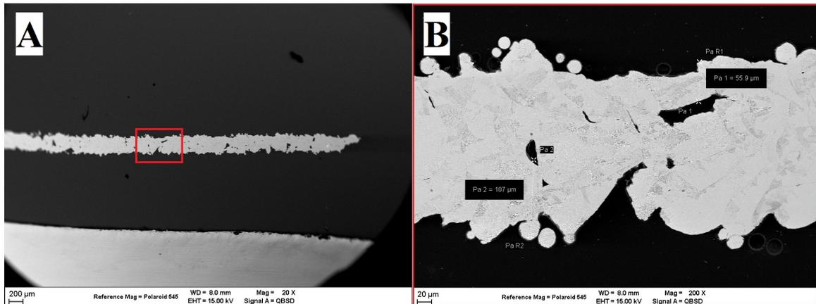
Figure 4: 0.25 mm Sample Built with Standard Parameters Imaged at x25 (A) and x200 (B)
