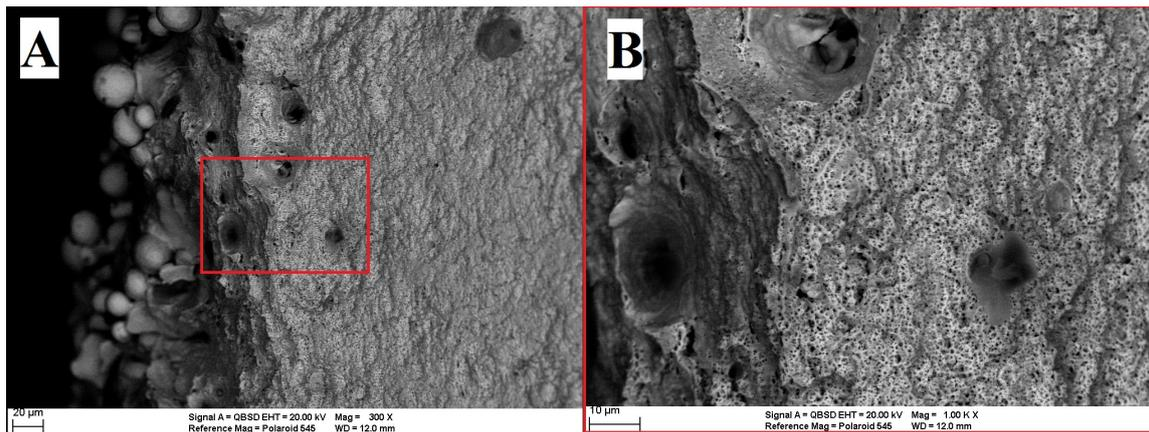
Figure 15: Fractography of 1.0 mm Sample with Compensated Scan Pattern Imaged at x300 (A) and x1000 (B) Showing Sub Surface Pores
