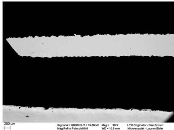
Figure 14: 1.0 mm Sample Built with Compensated Scan Pattern Imaged at x25
