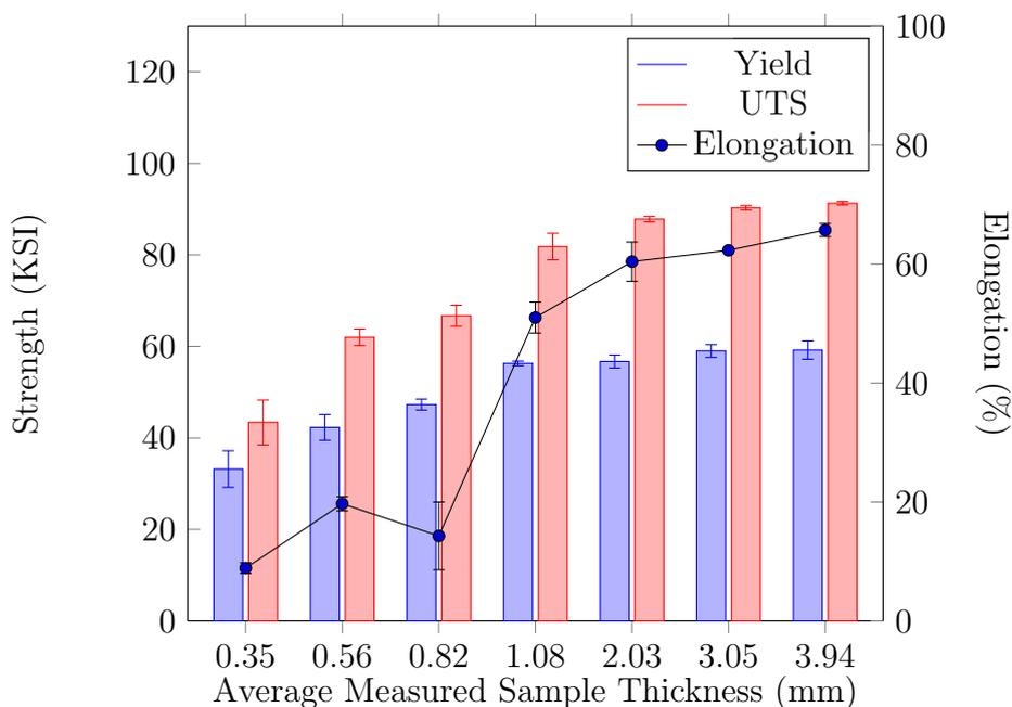
Figure 3: Mechanical Results for SLM 304L Standard Parameters
