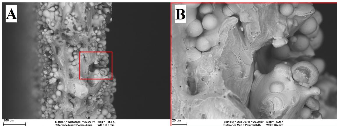
Figure 7: Fractography of 0.25 mm Sample Imaged at x151 (A) and x500 (B) Showing Surface Inconsistencies
