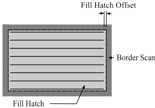
Figure 11: Schematic of Compensated AM250 Border Offsets
