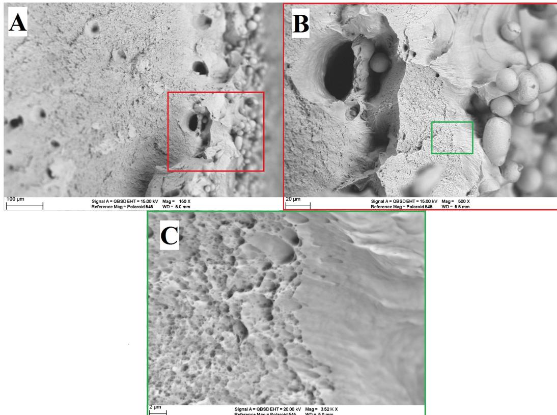
Figure 9: Fractography of 1.0 mm Sample Imaged at x150 (A) and x500 (B) Showing Subsurface Pores, and x3520 (C) Showing Shear Voids
