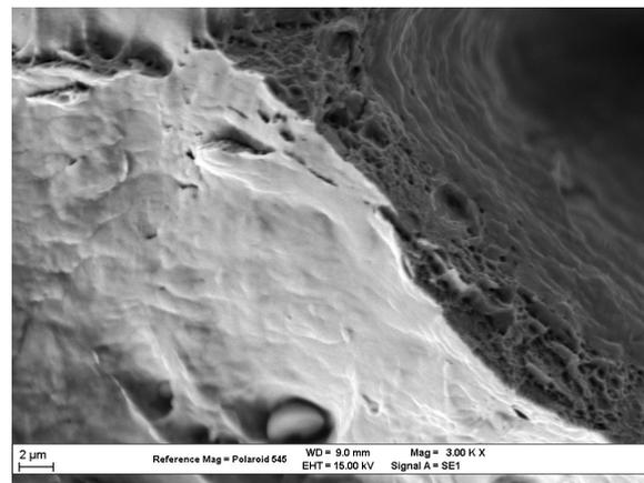
Figure 8: Fractography of 0.25 mm Sample Imaged at x3000 Showing Microvoid Coalescence and Shear Failure
