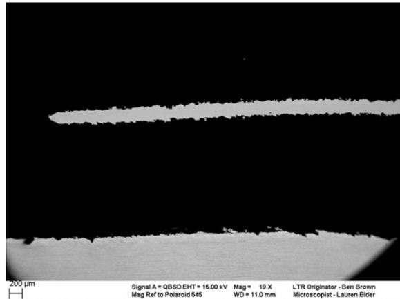
Figure 13: 0.25 mm Sample Built with Compensated Scan Pattern Imaged at x25
