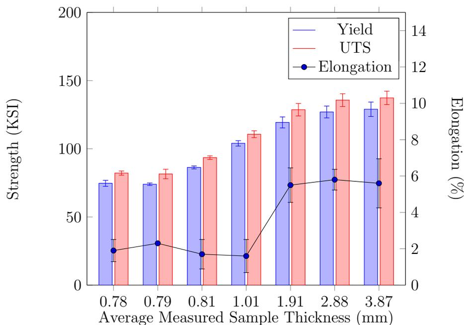
Figure 10: Mechanical Results for EBM Ti-6Al-4V Standard Parameters
