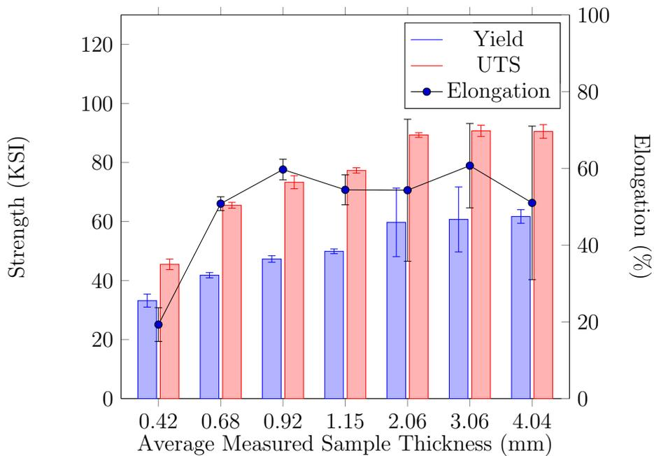
Figure 12: Mechanical Results for SLM 304L Compensated Parameters
