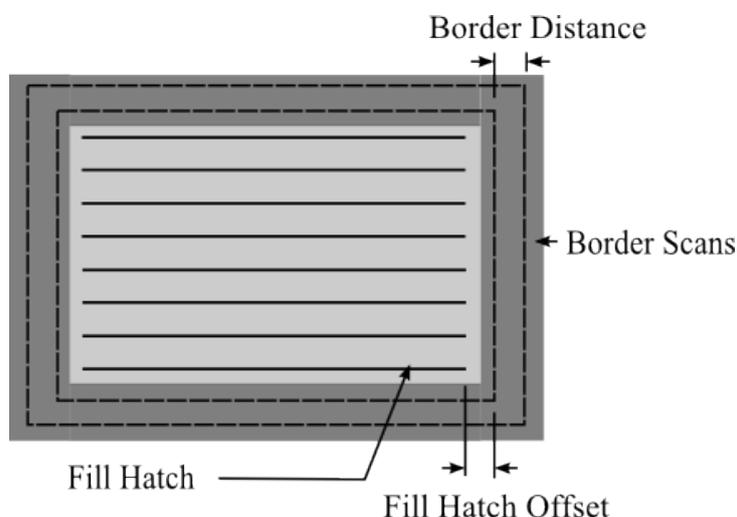
Figure 2: Schematic of the AM250 Border Scan Offsets for one layer the Standard Parameter Set
