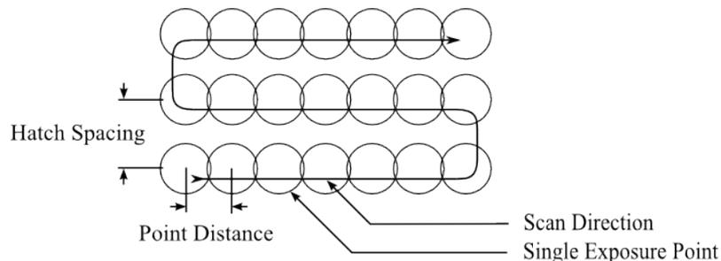
Figure 1: Schematic of the point wise AM250 Hatch Fill Scan Pattern
