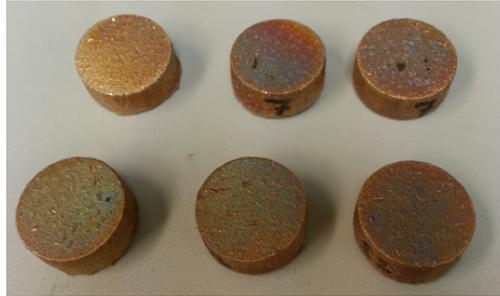
**Figure 8** Disks Prior to Finish Machining
