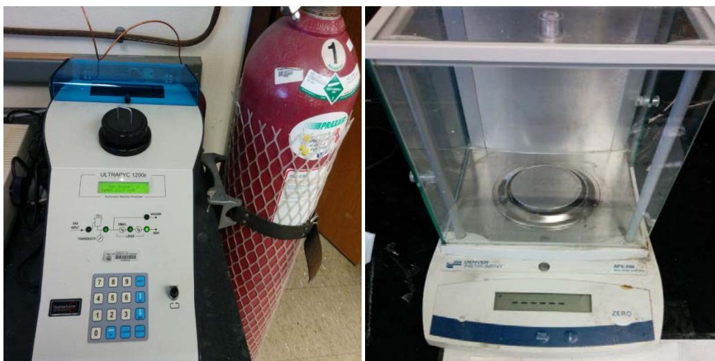
Figure 6. a) Ultrapyc 1200e Helium Pycnometer b) Denver Instrument Weightometer APX 200
