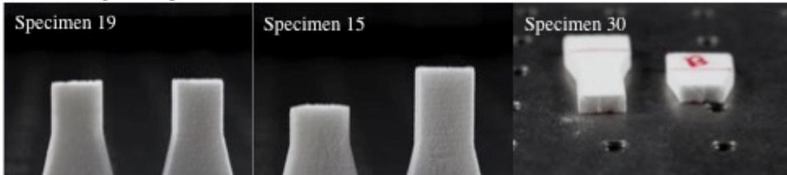
Figure 17 - Sample fracture images for low and high strength specimens
