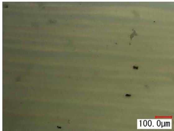
Fig. 10 Cross section of a part with 96% of part density
