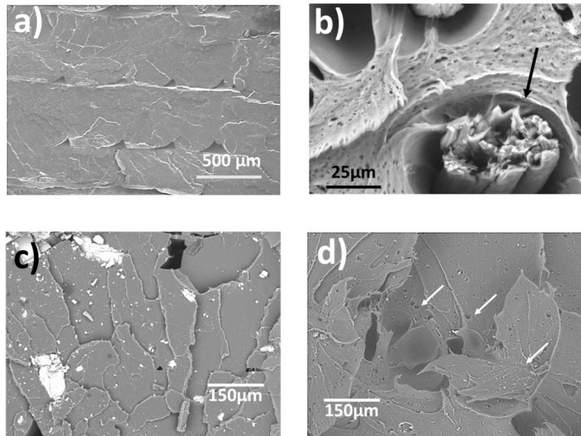
**Fig. 2. SEM Micrographs of materials tested in this study: a) PLA; b) PLA/jute plant fiber; c) PLA NaCl; and d) PLA/MayaCrom® Blue.**
