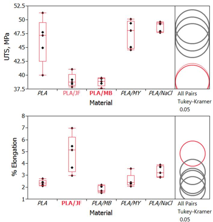
**Fig. 1. Tensile test results of materials tested here.**
