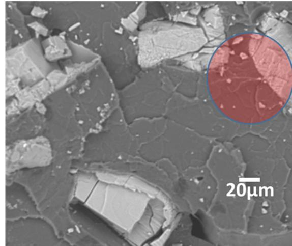
**Fig. 3 NaCl adhered well to the matrix and exhibited a robust interface and shared crack propagation features with the matrix.**
