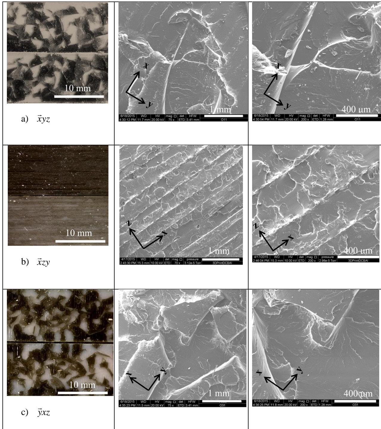
**Figure 9.** Failure surfaces and SEM images of Al-DCBs printed in the a)  $\bar{x}yz$ , b)  $\bar{x}zy$ , and c)  $\bar{y}xz$  orientation.
