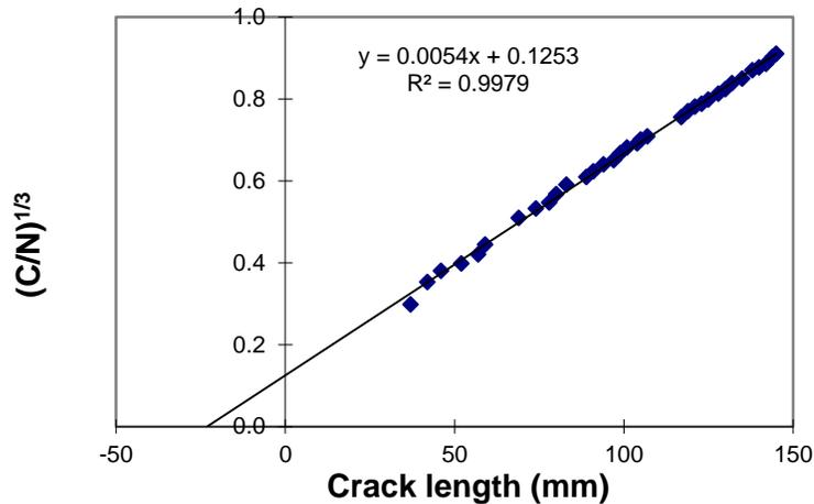
**Figure 3.**  $(C/N)^{1/3}$  vs. crack length  $a$  for aluminum DCB at 1 mm/min
