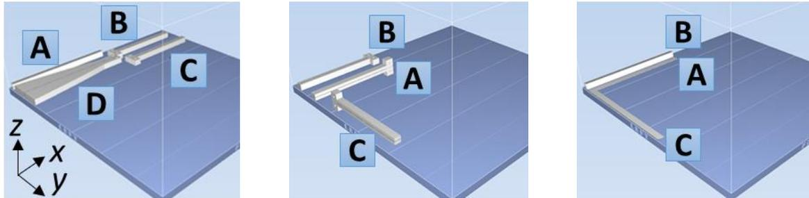
**Figure 2.** Illustration of various print orientations used to fabricate specimens. *Left:*  $xyz$  orientation for A) 3D printed (3DP) sandwich strips, B) and C) FP-DCB, and D) TDCB specimens. *Middle:* fully-printed DCB specimens oriented A)  $xyz$ , B)  $xzy$ , and C)  $yxz$ . *Right:* Al-DCB specimens oriented A)  $xyz$ , B)  $xzy$ , C)  $yxz$ .
