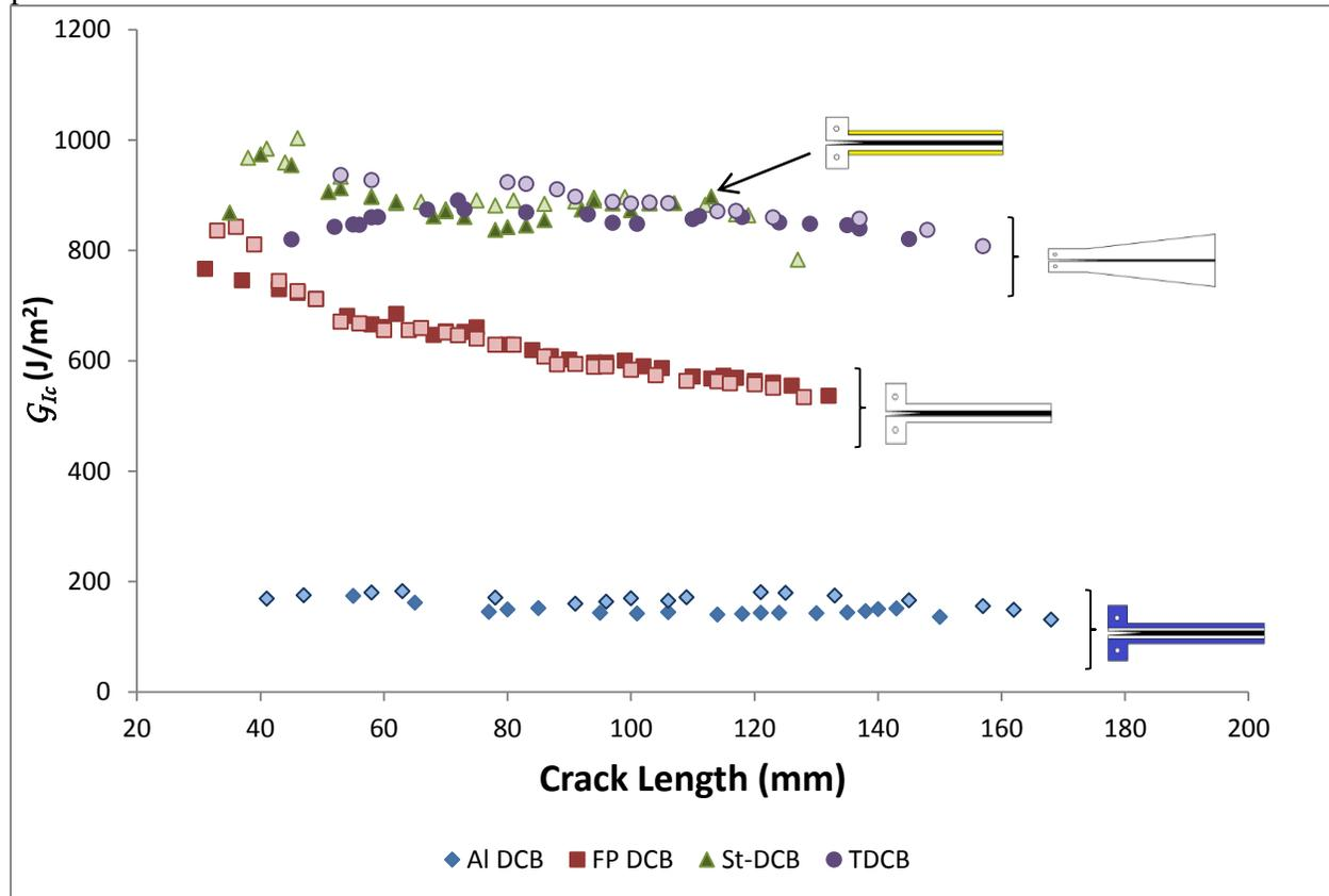
Figure 4 shows the variation of mode I fracture energy for all specimens, where two tests were conducted for each specimen type, with good consistency of the replicates.
