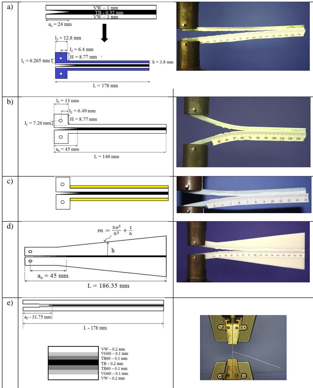
**Figure 1.** Illustrations of test configurations and photos of representative specimens during testing. Top to bottom are a) the aluminum-supported (AL-DCB), b) fully-printed (FP-DCB), and c) steel-backed DCB (St-DCB), d) TDCB, and e) T-peel geometries.
