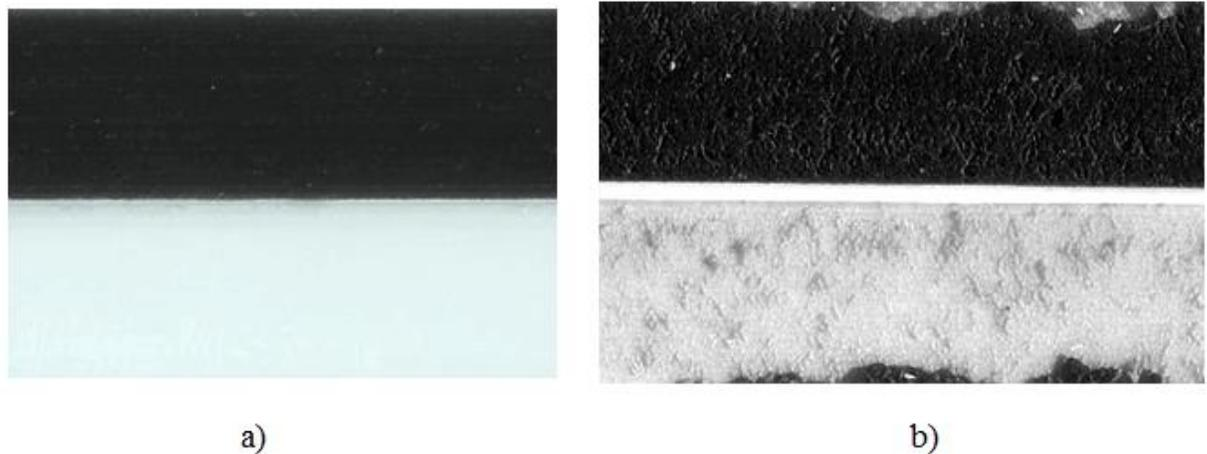
**Figure 13.** Failure surface of T-peel specimens. a) TB/VW and b) gradient
