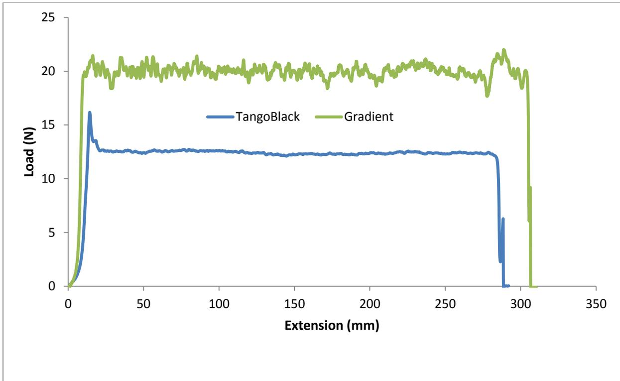
Figure 12. Load vs. extension curves from T-peel tests
