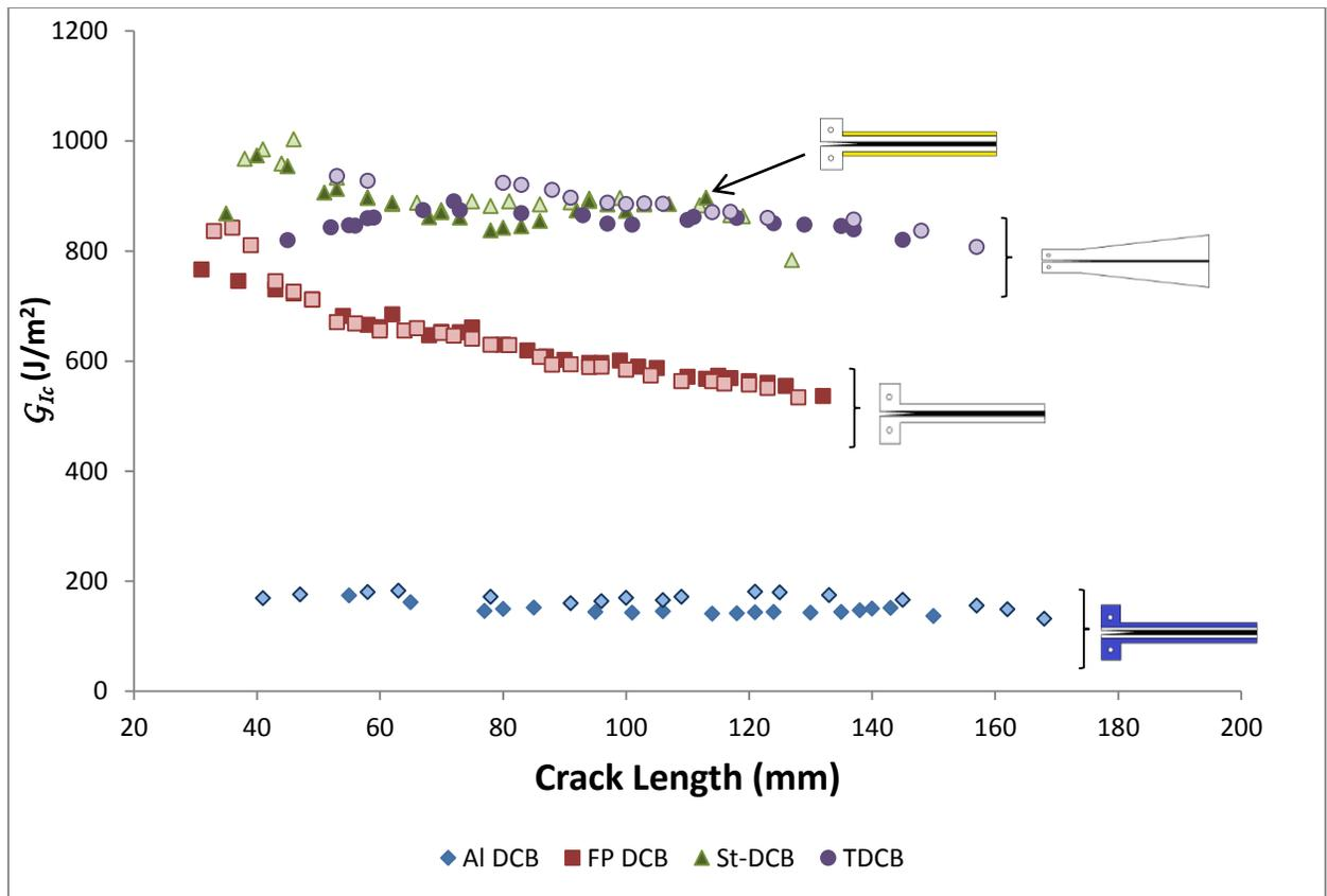
**Figure 4.**  $G_{Ic}$  vs. crack length for all DCB configurations in the  $\bar{x}zy$ -orientation: blue diamonds (AL-DCB), red squares (FP-DCB), green triangles (St-DCB), and purple circles (TDCB).
