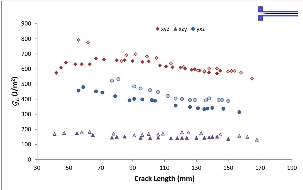
Figure 8.  $G_{Ic}$  vs. crack length for the Al-DCB configurations based on orientation.
