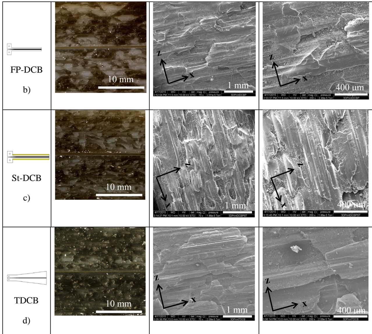
**Figure 5.** Failure surface of specimens with corresponding SEM images. Plane of the interlayer is oriented on the xz plane, with the direction of crack propagation aligned along the x axis
