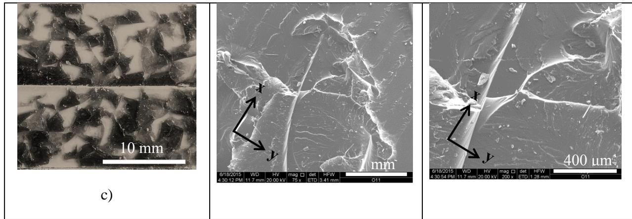
**Figure 11.** Failure surfaces and SEM images of Al DCB printed in the  $\bar{x}\bar{y}\bar{z}$  orientation and tested at the displacement rate of a) 0.01 mm/min, b) 0.1 mm/min, and c) 1 mm/min
