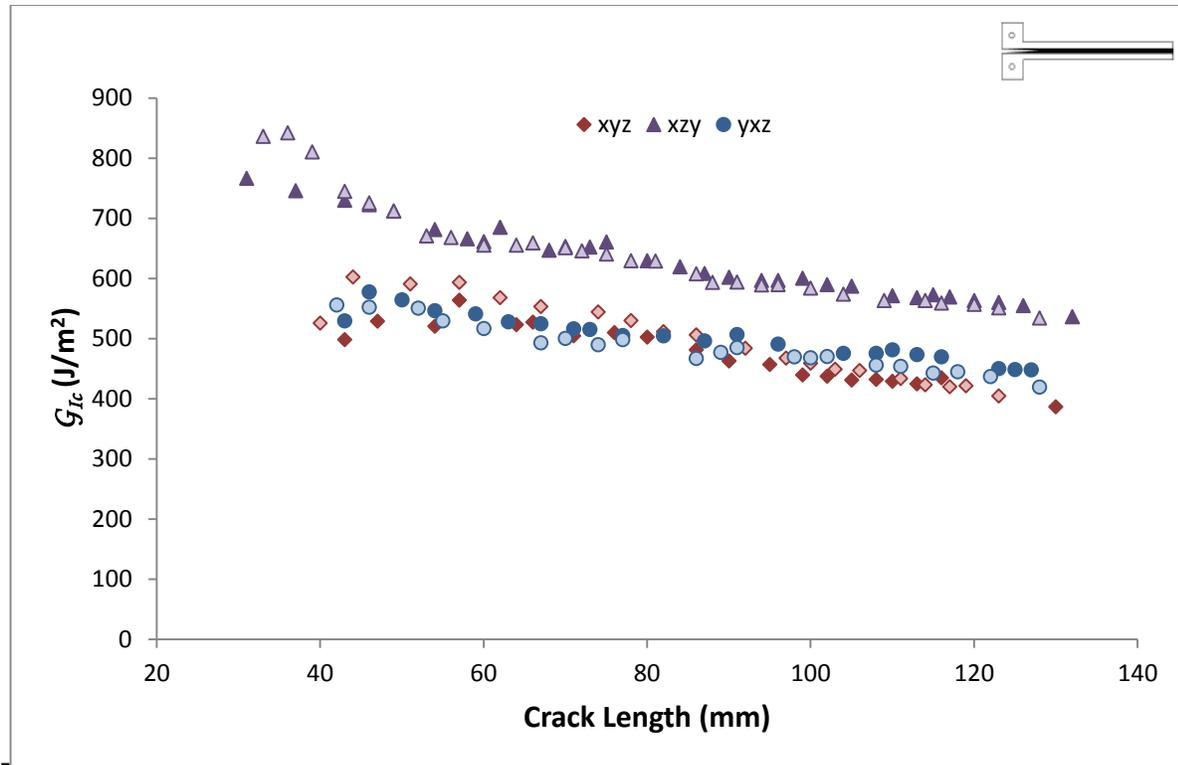
**Figure 6.**  $G_{Ic}$  vs. crack length for the fully-printed DCB configurations based on orientation
