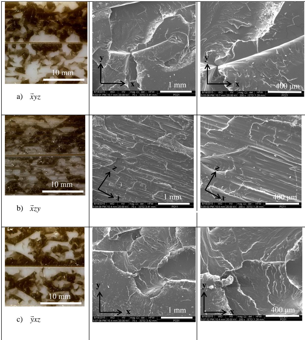
**Figure 7.** Failure surfaces and SEM images of fully printed DCBs printed in the a)  $\bar{x}yz$ , b)  $\bar{x}zy$ , and c)  $\bar{y}xz$  orientation.
