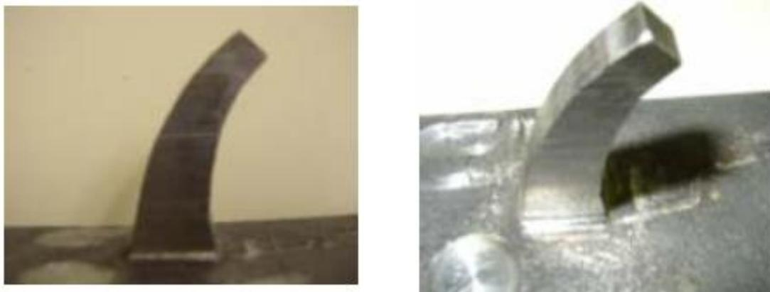
Figure 6 Picture of a part produced by a 5 axis Hybrid Manufacturing machine [26]
