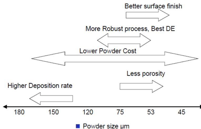
Figure 1 A graph detailing the merits of different particles size distributions of powder in blown powder DED [9].
