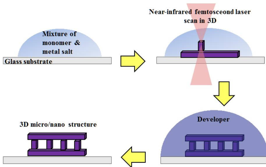
**Figure 1:** Illustration of fabrication steps.
