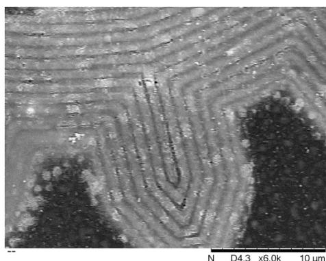
**Figure 3:** SEM image of SU8-Au nano-composite. The grey lines were made of SU8, and the white dots embedded in the grey lines were Au nanoparticle aggregations.
