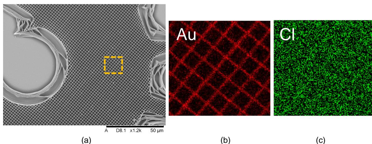
**Figure 5:** (a) SEM image of IPL-Au nano-composite fabricated using rhodamine B as an extra photoinitiator. The pattern is about 10  $\mu$ m high, with 25 layers. (b) & (c) EDX mapping analysis showing Au and Cl distribution in the area marked in figure (a), which proved that gold chloride has been successfully reduced into gold.
