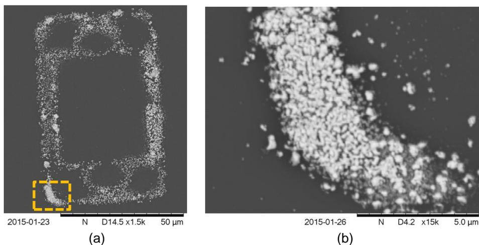
**Figure 4:** (a) SEM image showing the fabricated pattern using the mixture of IPL with gold chloride without extra initiators; (b) Magnified SEM image showing the section marked in figure (a).
