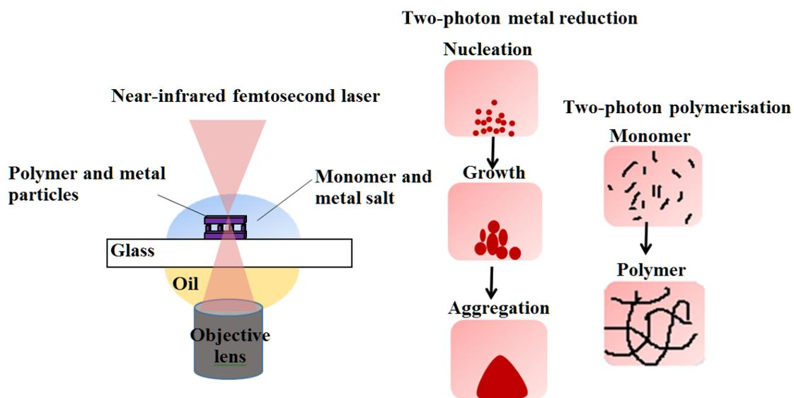
**Figure 2:** Illustration of fabricating nano-composites in a single step by two-photon induced polymerisation and metal salt reduction
