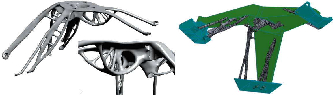
Figure 8: a) Final RW-Bracket Design b) comparison of conventional and AM design
