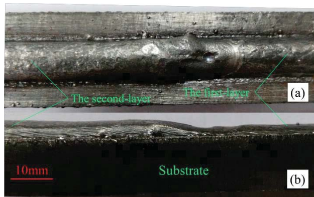
Fig. 4 The unfinished weld bead of second-layer deposition of the single-pass thin-walled part: (a) top view; (b) front view.
