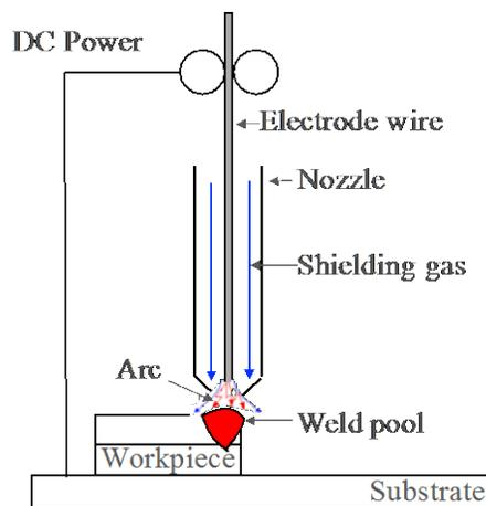
Figure 2. Schematic of gas metal arc welding.
