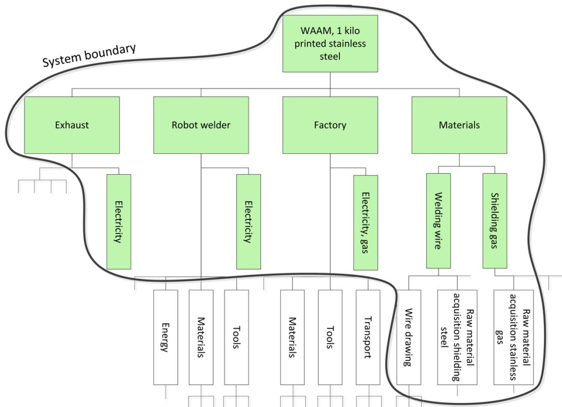
Figure 3. System Boundary of the WAAM process.
