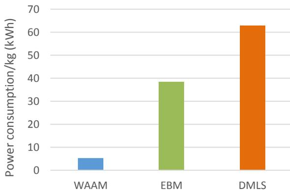
Figure 7: Power consumption per kg of metal by WAAM, EBM, and DMLS.
