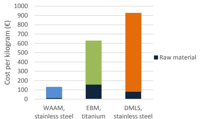
Figure 8: Cost estimation per kg of metal by WAAM, EBM, and DMLS.
