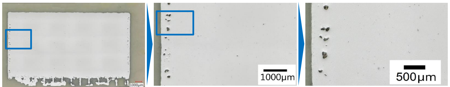
Figure 5: Cross section of density cubes (standard oxygen controlled atmosphere) for powder B
