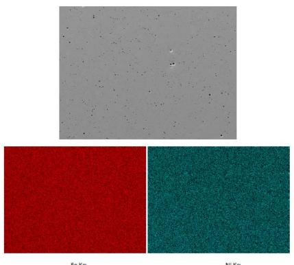
Fe Kα Ni Kα Figure 7. Gray scale image and colored EDS elemental map of a print made at 75% power and heat treated. The image is from the top.
