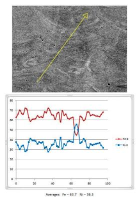
Figure 6. BEI gray scale image of a part printed at 100% power (side view) with line scan showing compositional variations across a random line in the microstructure.
