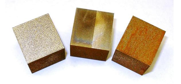
Figure 1. As-printed samples, nominally 20 mm per side. Left: top surface. Middle: bottom surface (after EDM removal from build plate). Right: side surface.
