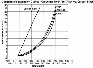
Figure 9. A plot of variation in CTE vs. Temperature for Invar  $36^{\text{(8)}}$  (6).
