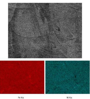
Figure 5. Gray scale image and colored EDS elemental map of a print made at 100% power. The image is from the side.
