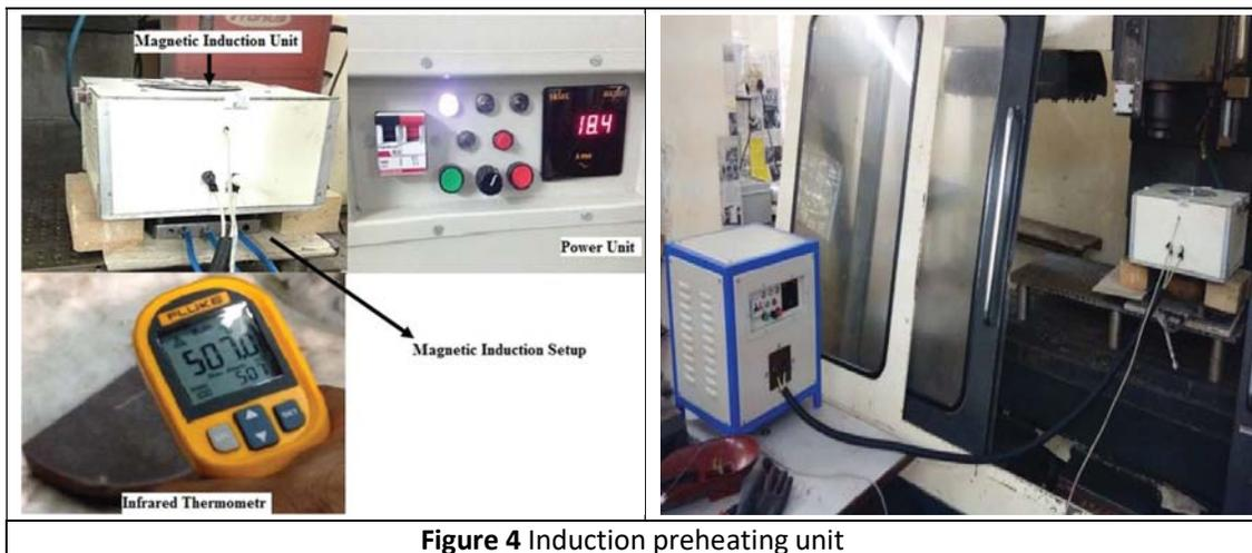
The 350<sup>0</sup>c and above preheating temperature maintained while layer by layer deposition was done. In the development of the tooling element using H13 tool steel material deposition
