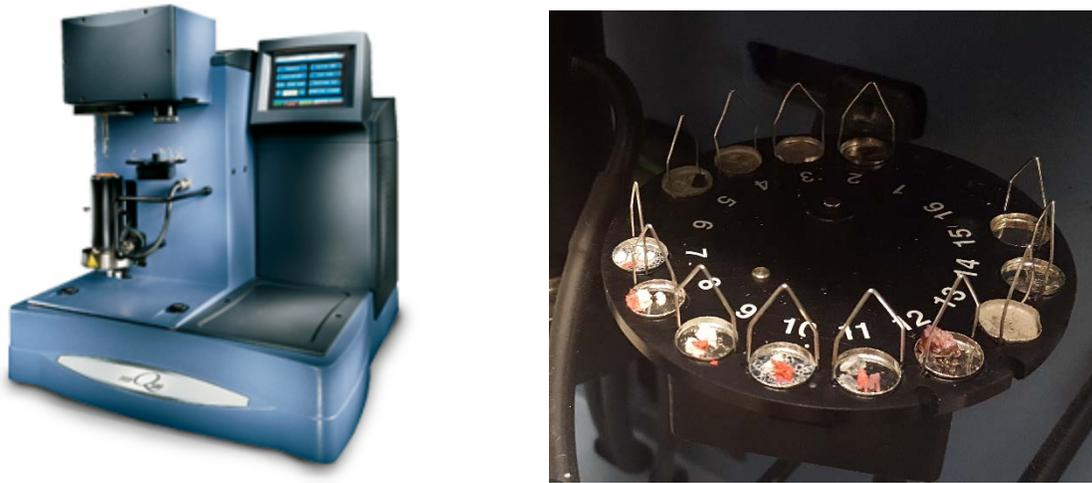
**Figure 6.** (Right) Universal Analysis Q500 TGA system [4]. (Left) Samples in TGA pans
