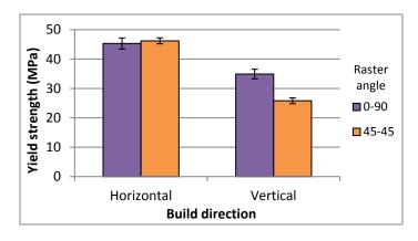
Figure 12. Effect of raster angle for horizontal-build and vertical-build sparse specimens
