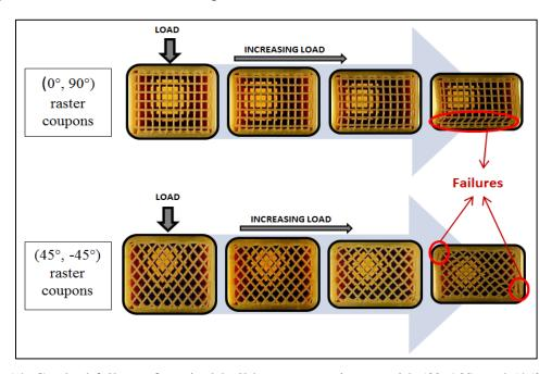
Figure 14. Gradual failure of vertical-build sparse specimens with (0°, 90°) and (45°, -45°) raster angles in compression tests
