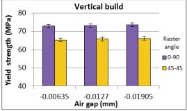
Figure 6. Interaction of build direction and raster angle on yield strength of solid specimens
