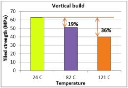
Figure 4. Decrease in yield strength of horizontal-build and vertical-build solid specimens
