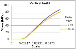
Figure 7. Sample compression stress-strain curves for horizontal-build and vertical-build solid specimens (air gap = -0.00635mm)
