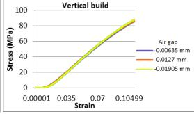
Figure 11. Stress-strain curves at different air gaps for horizontal-build and vertical-build specimens, where the raster angle was (0°, 90°)
