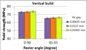
Figure 10. Effect of air gap on yield strength for solid specimens
