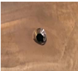
(a) A hole defect on component
