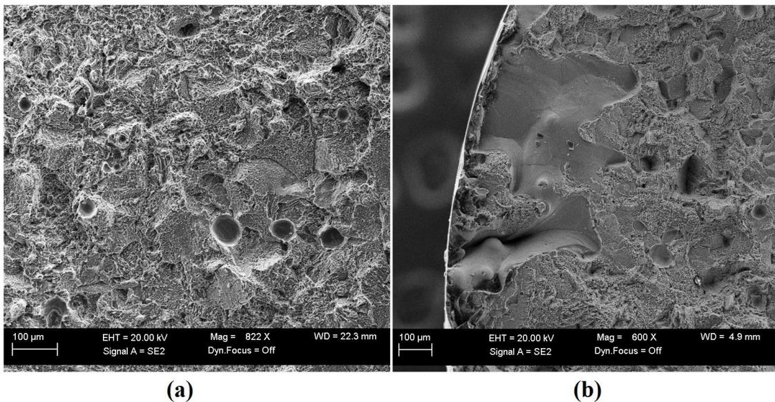
Figure 5. Pores from tensile fracture surfaces of (a) a single built LENS, and (b) a double built LENS Ti-6Al-4V specimen.
