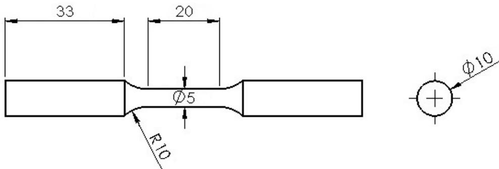
Figure 1. Dimensions of cylindrical tensile fatigue specimens based on ASTM E606 (units in millimeters).
