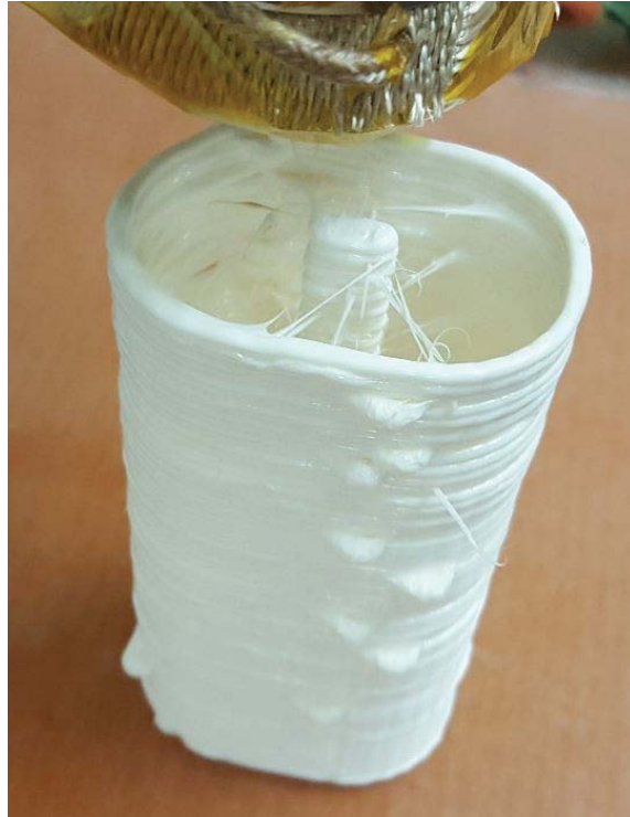
Figure 11: Z specimen as printed. The stacked skirts allow the nozzle to clear while also supporting the specimen
