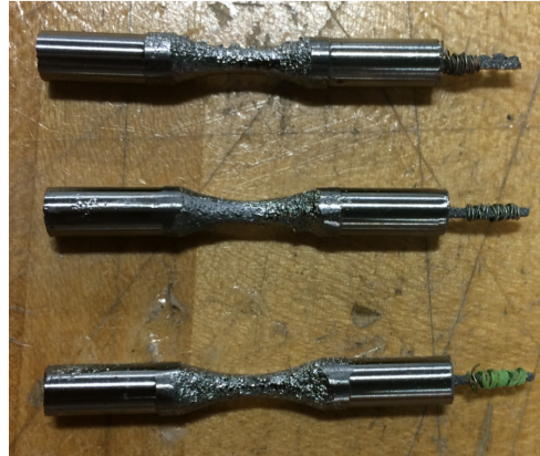
Fig.12 Electropolished fatigue samples after machining
