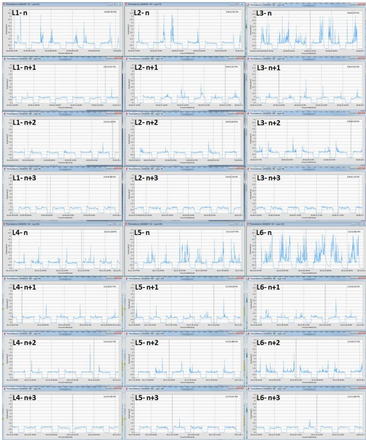
Figure 7. Data collected from photodetector from the six levels of contamination with tungsten. Four layers per contamination level are studied.
