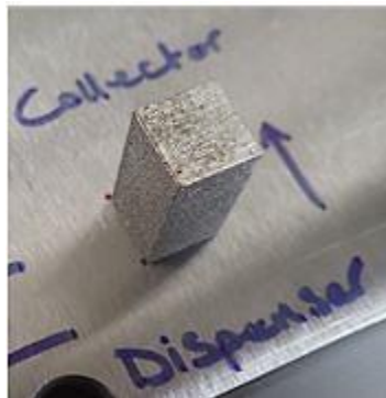
Figure 3. A rectangular specimen made of Inconel 625, containing contamination layers.
