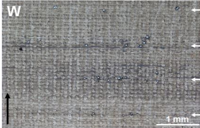
Figure 8. Low magnification optical images of the specimens contaminated by tungsten. The white arrows indicate the contamination deposition layers. The black arrow indicates the buildup direction.
