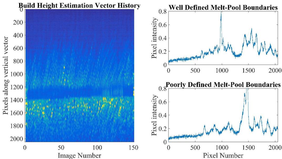
Figure 6. Pixel intensities along build height search vector over time (left). Examples of a well-defined set of height boundaries (top-right) compared to a set of poorly-defined boundaries (bottom-right) for the same scan speed and laser power settings.
