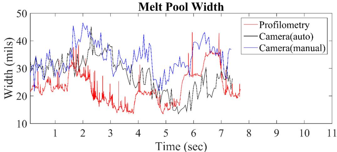
Figure 9. Comparison graph of melt-pool width obtained from measurements of manual boundaries, algorithmic boundaries, and optical profilometer data.
