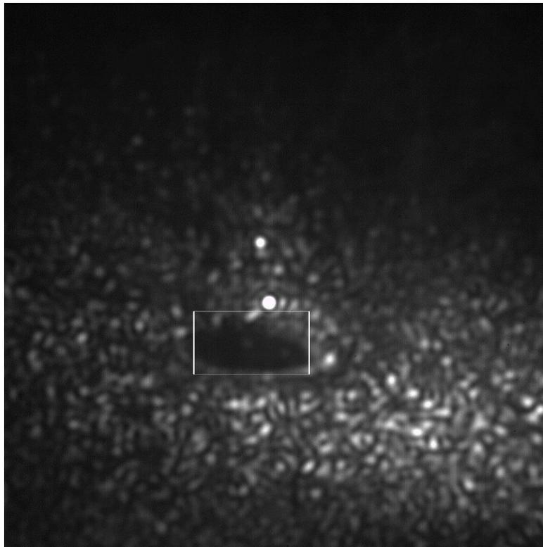
Figure 5. Camera image at time 2.5 seconds during second set of experiments with build height and melt-pool width parameter box drawn as estimated by melt-pool geometry algorithm.
