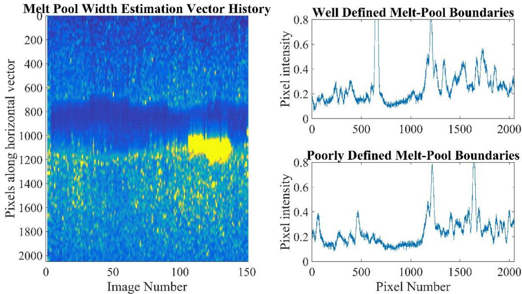
Figure 7. Pixel intensities along width search vector over time (left). Examples of a well-defined set of width boundaries (top-right) compared to a set of poorly-defined boundaries (bottom-right) for the same scan speed and laser power settings.
