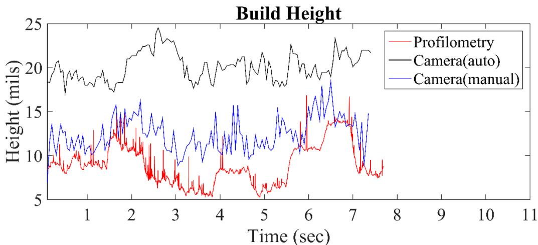
Figure 8. Comparison graph of build height obtained from measurements of manual boundaries, algorithmic boundaries, and optical profilometer data.
