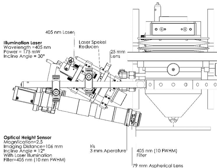
Figure 1. Camera and initial illumination system mounting fixture.
