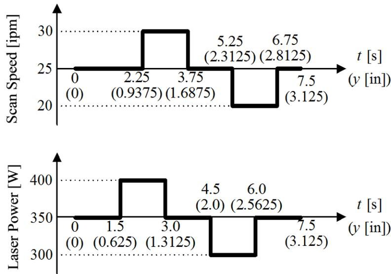
Figure 2. Laser Power and Scan Speed input commands for experiments.
