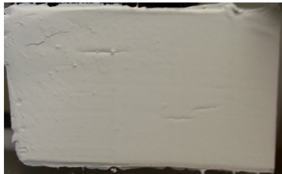
Figure 5. Cracks as a result of fast drying.
