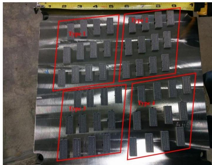
Fig. 5 samples on the multiple support structure patterns
