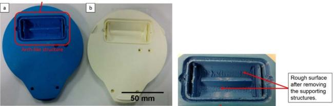
Figure 3. Comparison of FDM printed (a) and injection moulding (b) plastic part.
